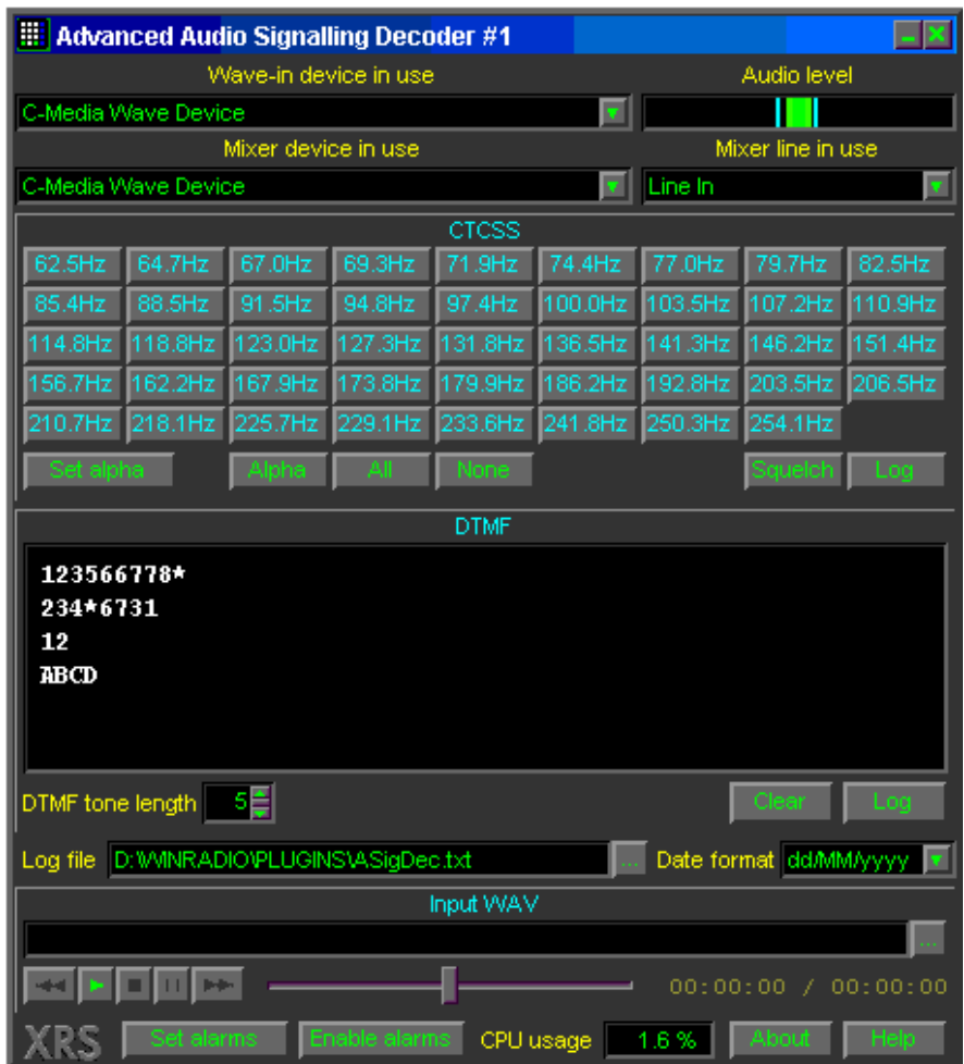
Advanced audio signaling decoder CTCSS and DTMF screen
